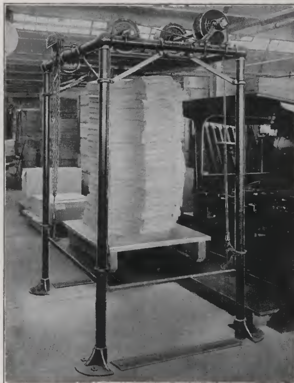
The Omaha Paper Hoist with Ratchet and Chain Hoist or fitted for Motor Drive.
