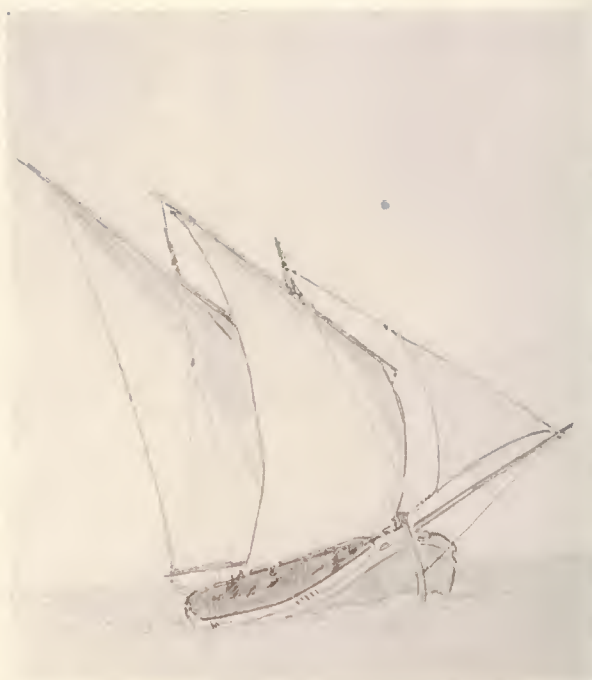
Greek schooner, lug rigged fore and main with a single small jib. These clumsy ships ply among the Greek Islands and to Egypt carrying fruit and vegetables. They are sturdy craft and need to be in the sudden storms from the north that come up in the Aegean.
