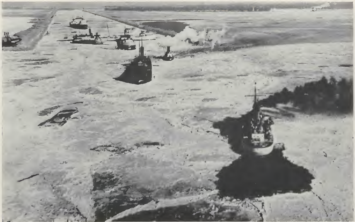
Coast Guard cutter Takoma breaking ice to free vessels frozen in the Detroit River.
