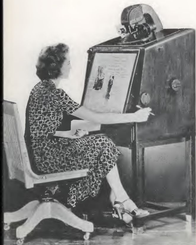
The film is run through the “reader” and enlarged to an ordinary type sized picture.
