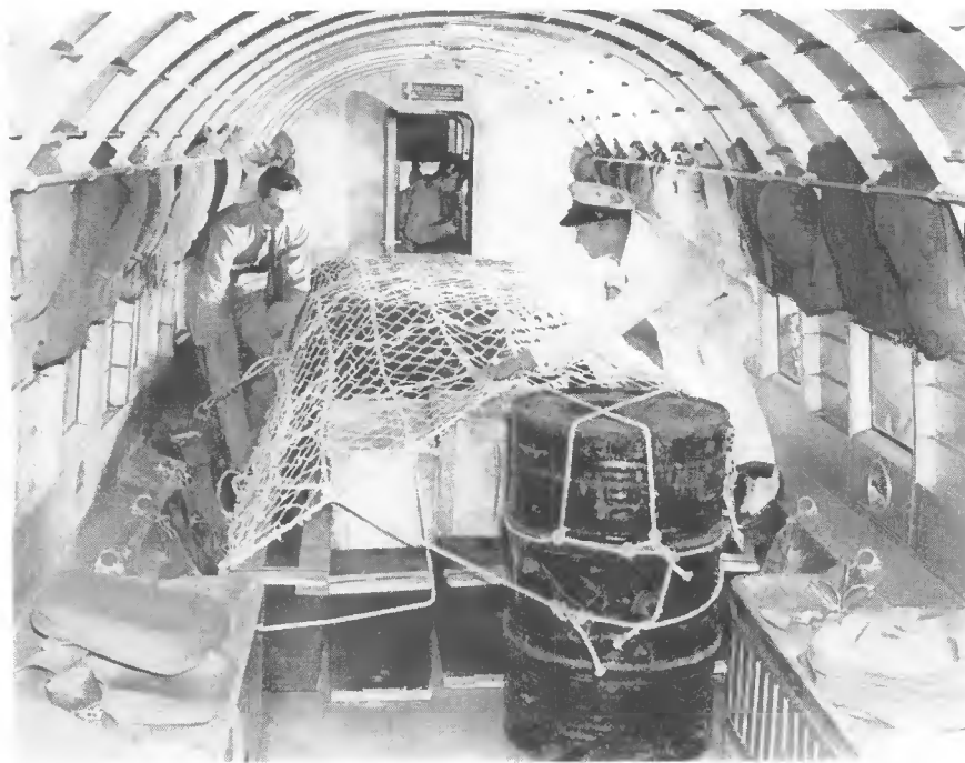
Douglas C-53 Interior view. Cargo plane is partially loaded with airplane tires, and drums of motor oil together with miscellaneous cargo.
