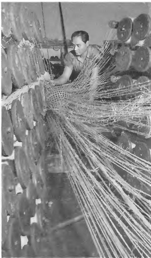
Tiny threads of abaca, or Manila hemp, twisted together make a ship's hawser in prewar Manila. GEOGRAPHIC photograph by J. Baylor Roberts.
