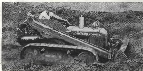
Willing worker for loading, clean-up work, grading and filling—a TD-6 and Bucyrus-Erie 3/4 yd. dozer-shovel.
