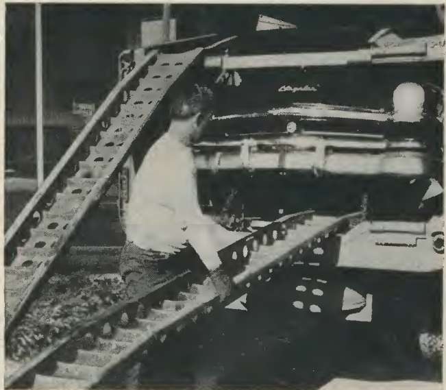
Strong as a bull . . . light as a calf. The heaviest cars must pass over these steel loading skids to get aboard giant auto trailers. The steel skids must be strong enough to support thousands and thousands of pounds yet be light enough for one man to handle. That's why many of them are made from strong, light-weight U-S-S COR-TEN Steel.
