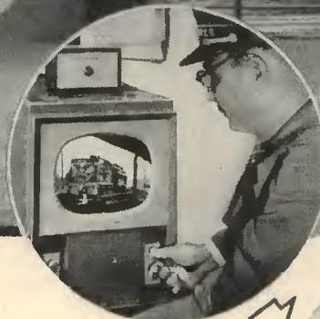
2. The visual information is fed by cable to a TV monitor at the station.
