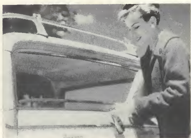
Roll-down rear window on all 1958 Rambler station wagons disappears into tail-gate. The one-piece cargo door eliminates upper hinges . . . gives more loading room.
