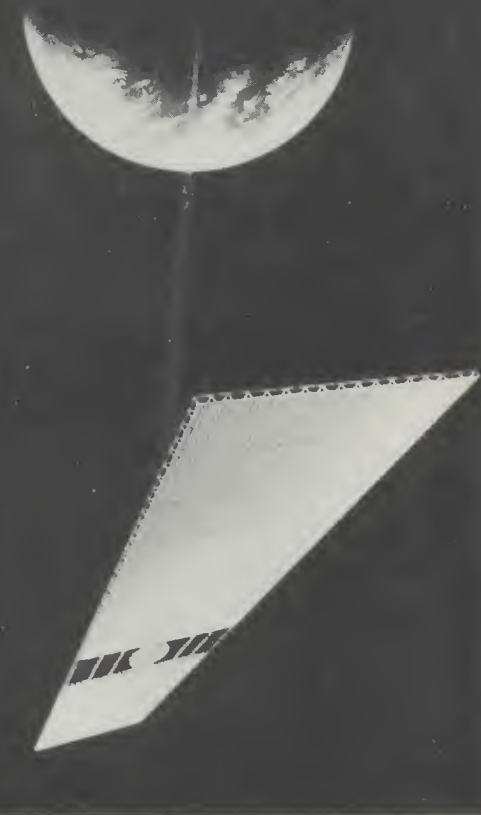
Artist's concept of proposed geosynchronous Space Solar Power satellite beaming microwave energy to earth for conversion into electric power.
